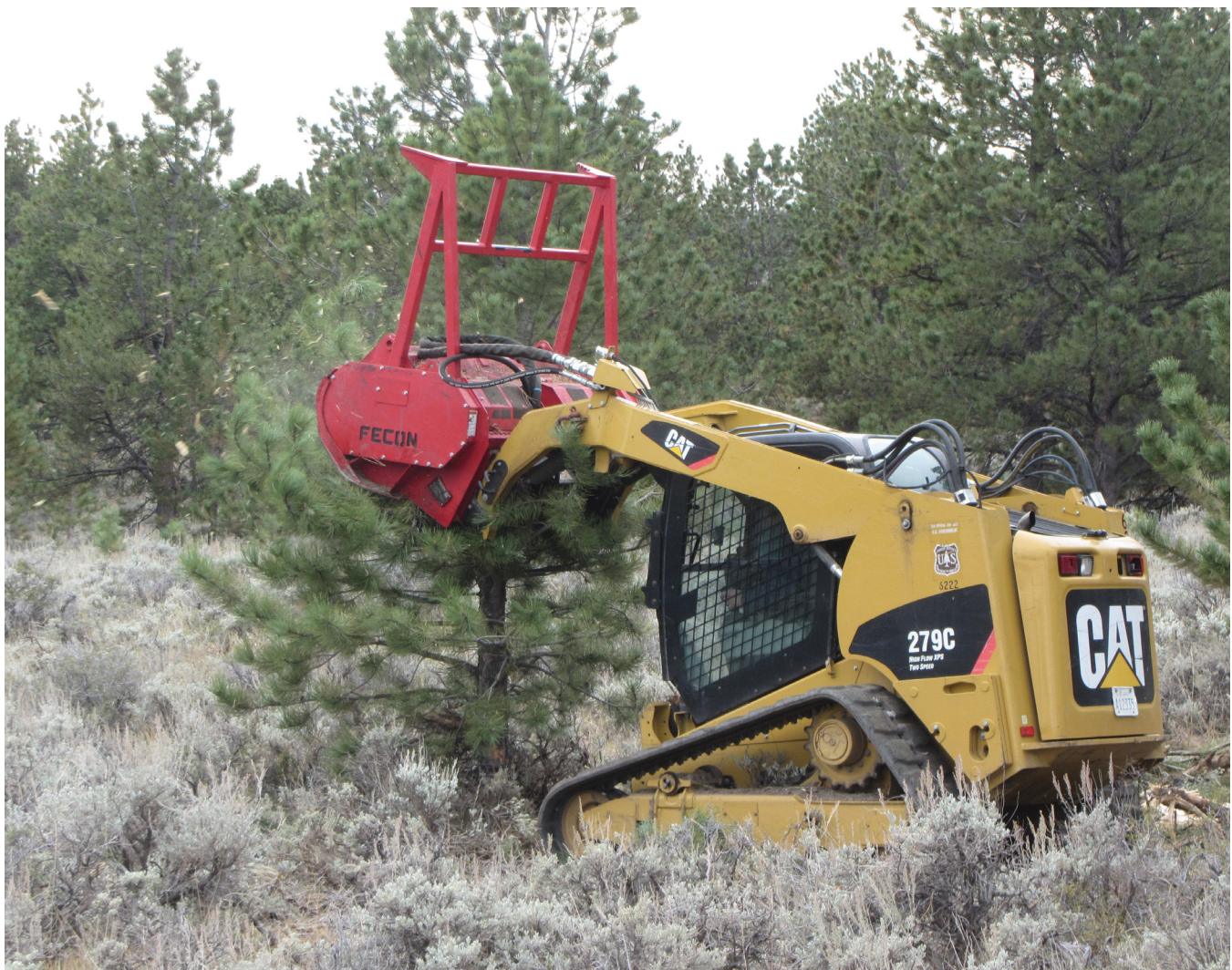
Figure 11. Mastication to manage conifer stand density in mixed forest-shrub-grassland systems. Photo Credit to Daron Reynolds.
